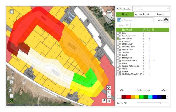
When moving along the surveyed area, keeping client device connectivity is desirable. Roaming allows moving devices to maintain wireless communication by connecting to new access points within the same network to maintain the quality of communication and prevent degradation of signal strength.
