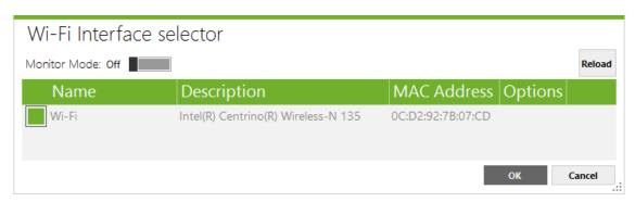
In **Acrylic Wi-Fi Heatmaps** you can use two different types of Wi-Fi devices, depending on their capturing capabilities. All commercially available Wi-Fi devices can be used to capture data on Native Mode. For extended capture capabilities, you will need a compatible wireless card to be used on Monitor Mode.
