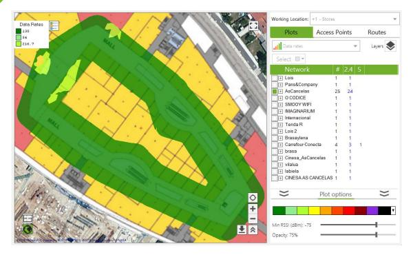
This transmission rate represents the maximum transmission rate supported by each access point. Even though an access point supports a certain maximum transmission rate, this maximum rate is not always achieved, due to noise in the radioelectrical medium, signal strength, number of client devices connecting the network, distance between access point and client device, etc. These factors can negatively impact the network's performance.
