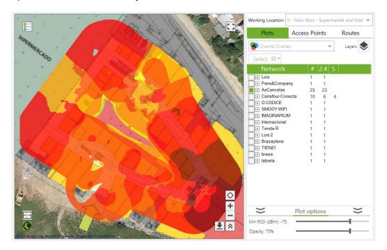
Adjacent channel interference is detected whenever a different access point is operating on an adjacent channel, causing transmission frequencies to overlap. This interference mostly depends on the channel bandwidth for each access point, and the signal strength differential (if lower than 20dBm).
